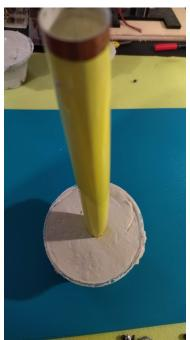
Fill a container with a thick mixture of plaster of Paris or better still MAP glue for placo. Coat the front of the warhead with WD 40, then push it in slightly, wait a few seconds then slowly pull it out.
