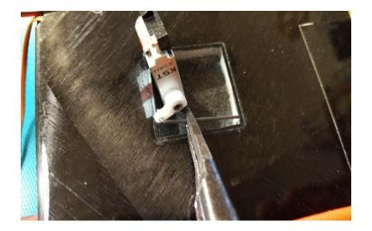
Prepare the epoxy resin + carbon powder mixture and fill the well of the bell cranks.
