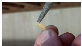
Reduce the size of the spreaders so that you only have the first hole, about 5 mm from the clamping screw.
