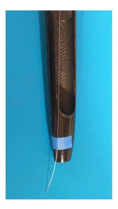
Make a loop and add a piece of cable in the crimp tube. Before disassembling the stab, all you have to do is tape this cable to the fuselage to prevent the control loop from falling into the tail tube!
