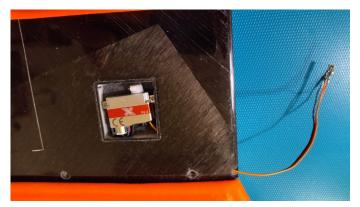
Take the servo and its support , pass the control rod through the wing following the original hole in the Rohacell, then fit the aileron control on the rudder.
