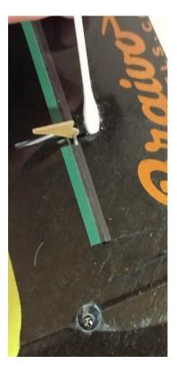
Installing control cables and rudder and stabilizer horns
