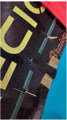
After cleaning the excess glue with a cotton swab soaked in alcohol, let the glue polymerize quietly.
