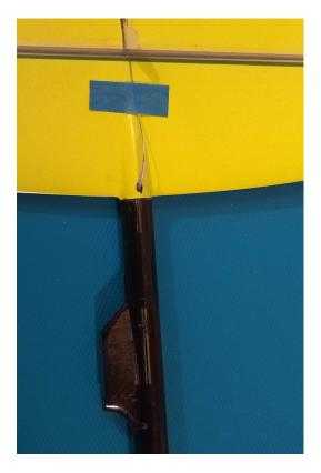
Tape the cable at both ends. Cut the elevator control cable to the correct length.
