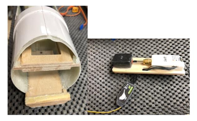
On the left pictures you can see the GPS drawer guide glued at the very end of the nosecone above and the fixture of the additionally buffer battery at the bottom. The used GPSequipment is placed on the plywood board.
