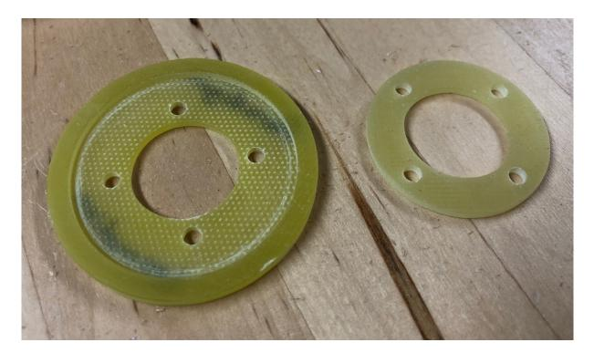
For the Leomotion motor it is necessary to put an 1.5mm GRP spacer inside the nosecone. Otherwise the gear of the Leomotion is too far outside the nosecone and the spinner will not fit close enough. I put epoxy on the spacer and fixed it with a 3mm steel pin in line with the motor holes.
