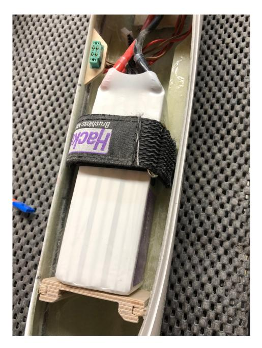
The Paradigm was also equipped for GPS flying. With the position of the battery directly behind the motor and thus above the controller, the area between the battery and the wing nose is available. This area is completely laminated from GRP without CFRP. The area is large enough to place the receiver forward and also to lay the receiver antennas inside the fuselage.
