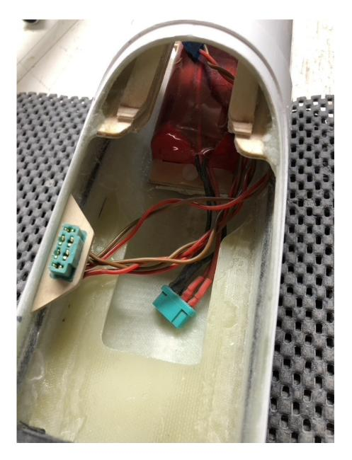
The buffer battery has found its place under the GPS equipment. The receiver is fixed to the buffer battery with Velcro tape and thus lies in the space between them. The receiver antennas are guided and fixed at an angle of 90° in bowden cable tubes on the plywood installations. The MPX connector for switching the buffer battery is placed in a plywood socket on the right inside of the fuselage.
